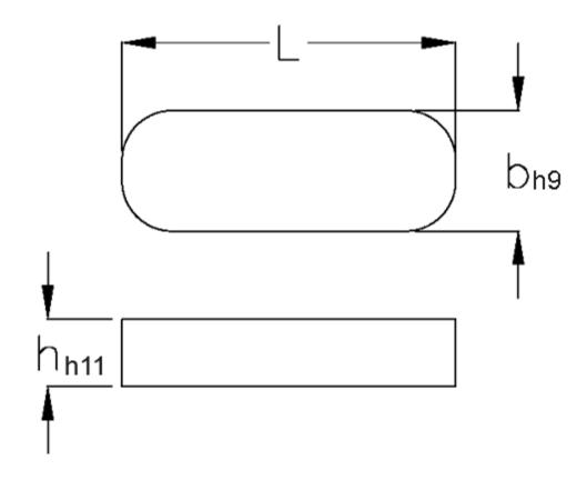
$\begin{array}{ll} b & = 32 \\ h & = 18 \\ L & = 110.0 \\ Tolerance \ b = 0.062 \\ Tolerance \ h = 0.110 \\ Tolerance \ L = -0.5 \end{array}$
